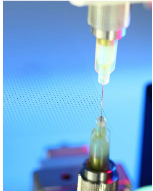
* i-DR S400 system enable micro-volume dispensing capability.
